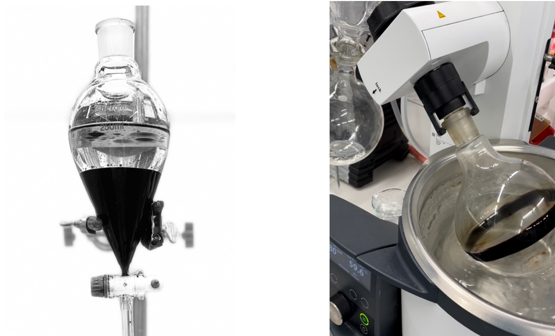
Figure 12: Representation of the process of liquid-liquid extraction and rotary evaporation
