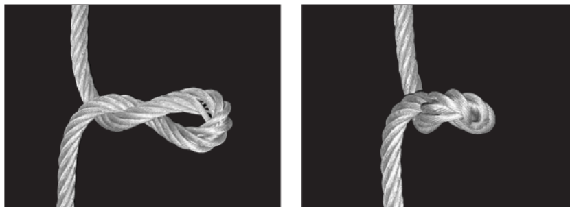
Figure 1.22: Damage to wire ropes because of hockling [51]
