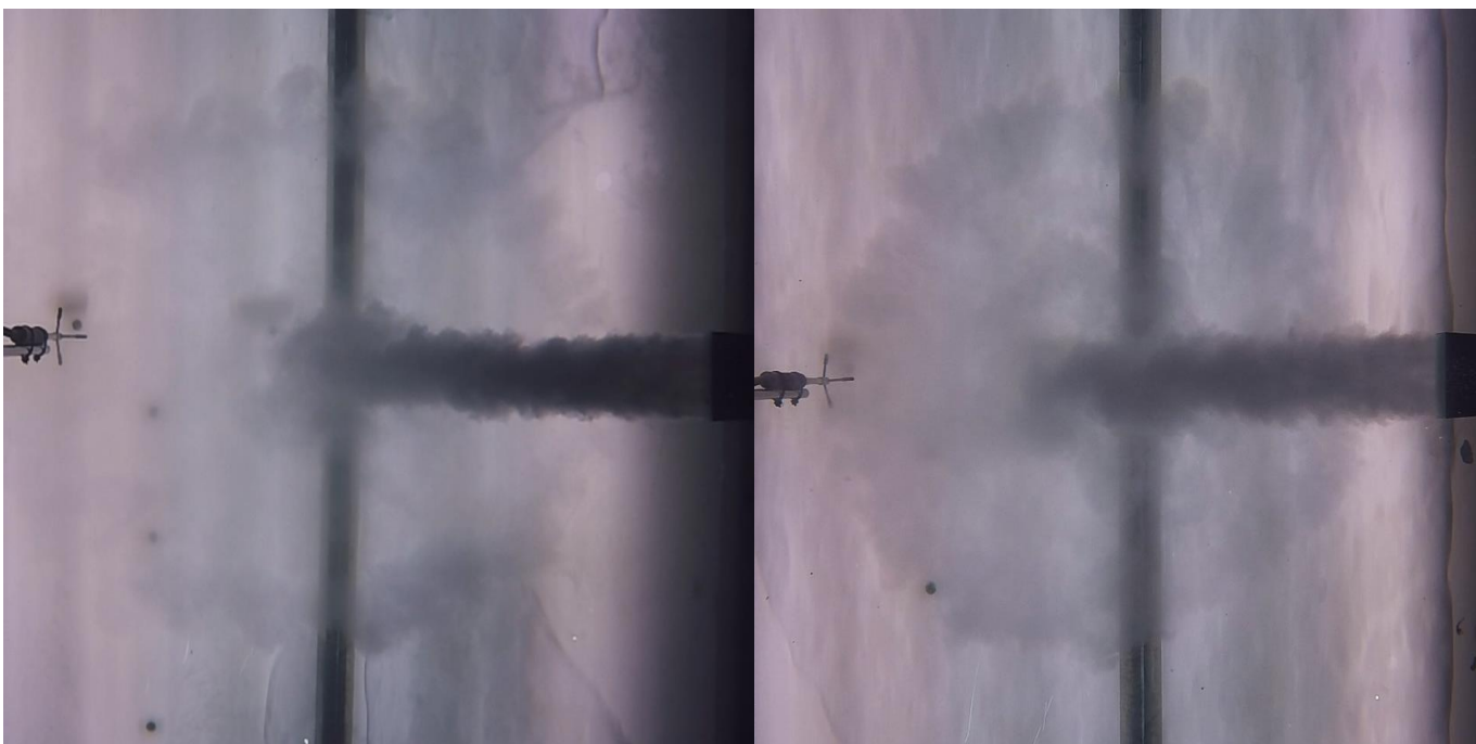
Figure 4.11: Stills from GoPro videos showing the outflow shape of the current the moment after first impingement for diffusers 1 and 2 respectively
