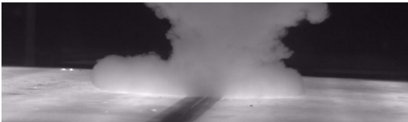
Figure 4.10: Still from the high speed camera recordings of diffuser 2, showing the initial horizontal spread just after impingement, associated with the increase in horizontal velocity as observed by the ADV as discussed in section 4.2.2.
