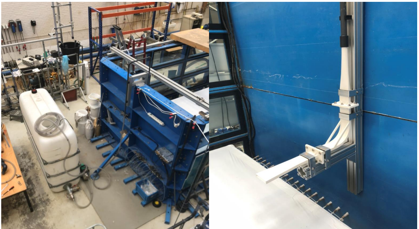
Figure 3.1: The left panel shows the mixing tank (white) and the modular tank (blue), connected by a flexible tube. The right panel shows diffuser 1 installed in the modular tank at a height of 30 cm above the table
