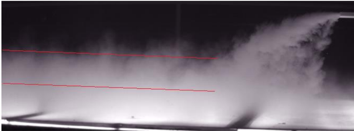
Figure 4.5: Still from the high speed camera recordings showing the steady-state of the flow from the diffuser. The region between the red lines is the height in the turbidity current associated with the low correlation, believed to be caused by Kelvin-Helmholtz instabilities.
