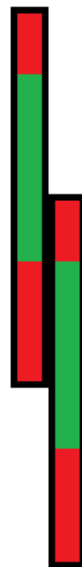
Figure 3.7: This schematic gives an impression of the overlap that will be applied to the measured profiles. The green area being the 'high accuracy' region, located between 5 and 20 mm as measured from the top of the profile, and the red being the area of which the values will be discarded
