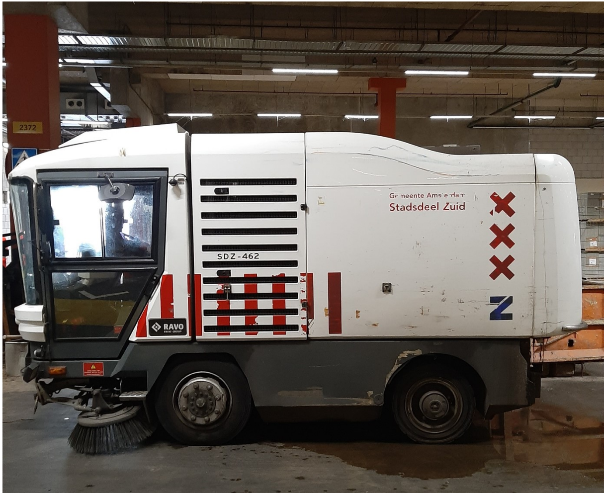
Figure 8 A RAVO street sweeper with in front of the brush the water sprayer. Interestingly, the text on this machine indicates that it belongs to Stadsdeel Zuid, a different area of the city of Amsterdam. This shows that machinery is shared between city areas
