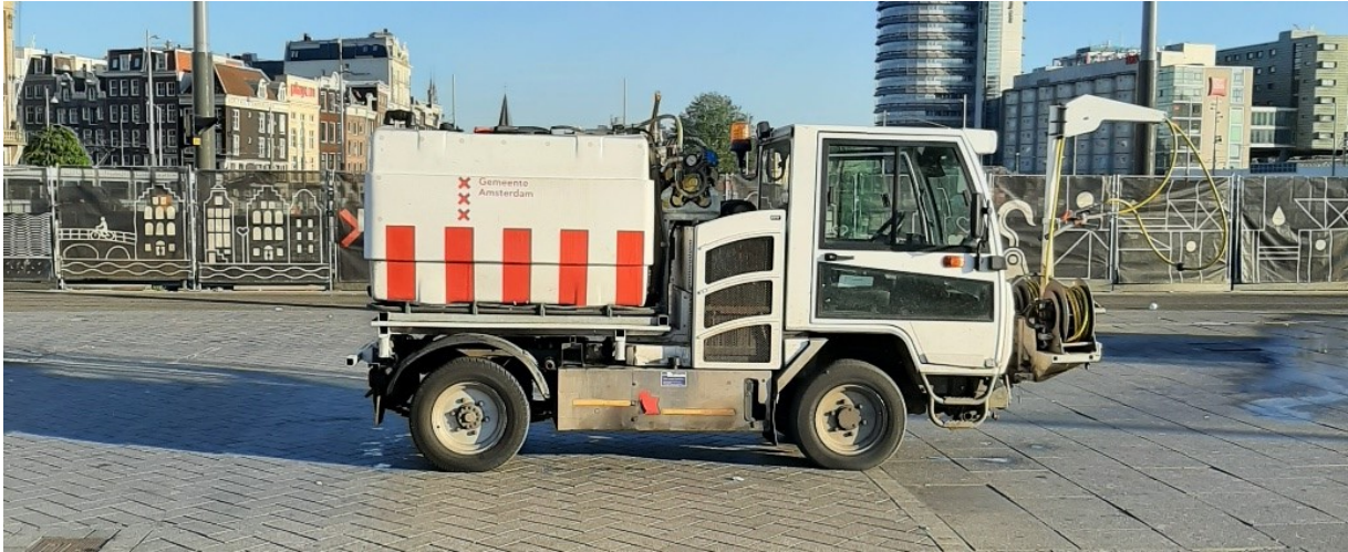
Figure 5 Spoelwagen used by the Schoon department equipped with high pressure sprayers
