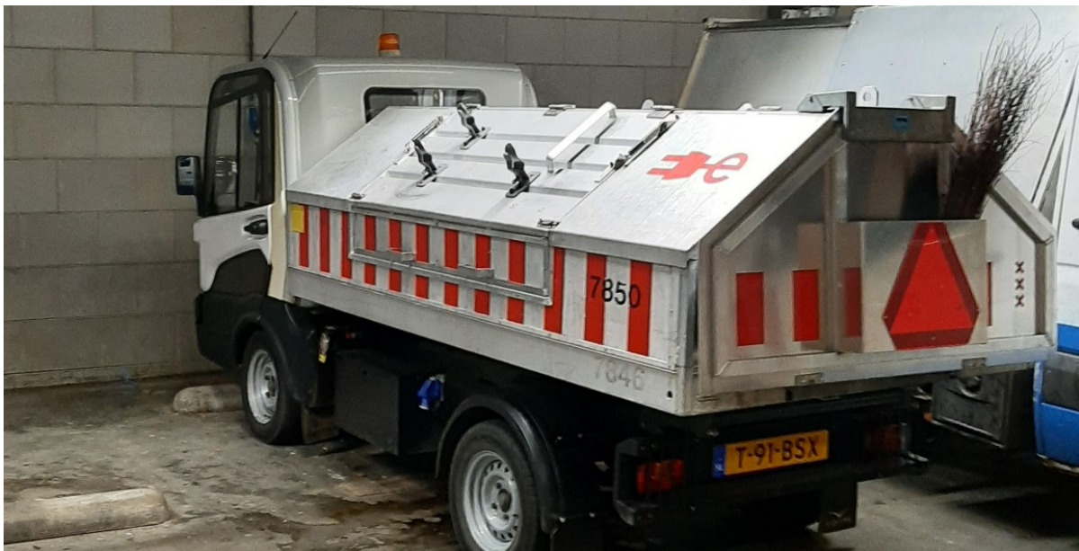
Figure 6 Goupil electric vehicle equipped with tipping system to access areas not accessible for normal vehicles
