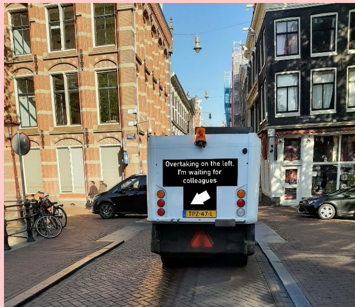
Figure 1310 The RobotRAVO indicating how bystanders can pass the vehicle
