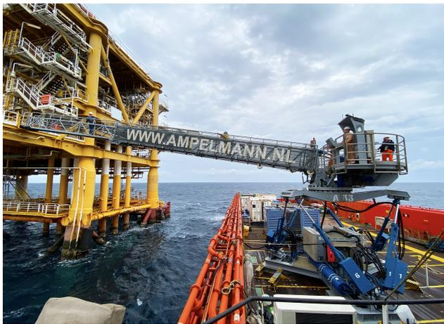
Figure 3.1: Ampelmann A-type crew transfer gangway (Ampelmann Operations B.V.)
