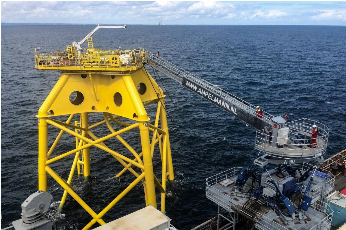
Figure G.1: Ampelmann A-type with conventional hydraulic actuators in operation.
