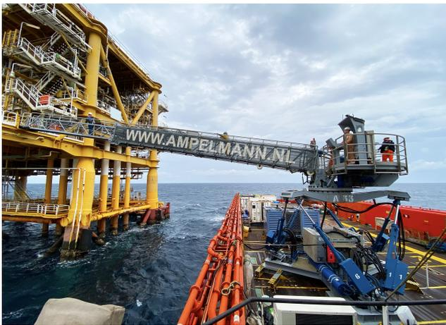
Figure 4.1: Ampelmann A-type crew transfer gangway (Ampelmann Operations B.V.)
