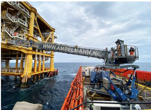
Figure 6.1: Ampelmann A-type crew transfer gangway (Ampelmann Operations B.V.)
