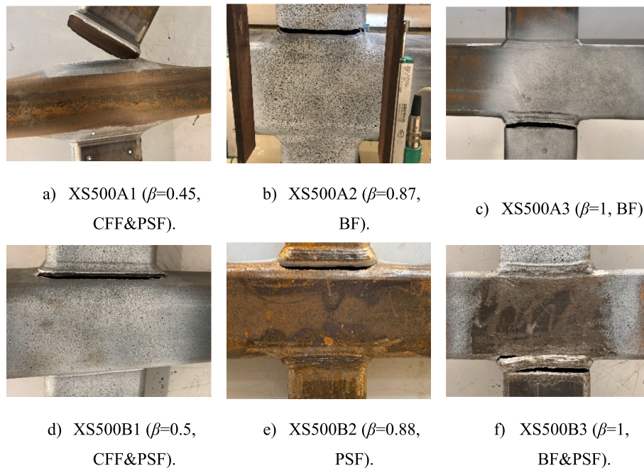
Fig. 9. Failure modes of S500 X-joints.
