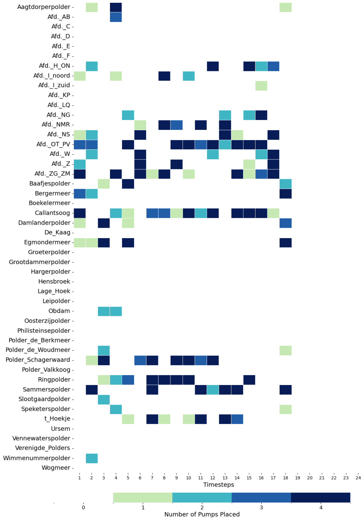
Figure 5.8: Pump count visualization for the five best solutions, showing pump placement for the five best solutions from table 5.1. The x-axis represents the timesteps (three hours per timestep). Instantaneous pump movement between polders is clearly visible. Also note that after timestep 18, no pumps are placed.
