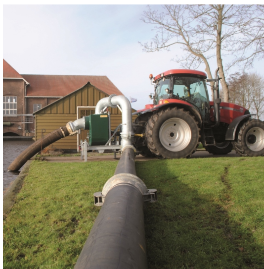
Figure 2.3: The BBA B300 centrifugal pump in operation [3]. The top pipe serves as the discharge side, while the suction side is located at the back. HHNK owns four pumps of this type. The pump is connected to the tractor via the transmission ( aandrijftras in Dutch). The discharge capacity also depends on the tractor's power.
