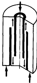
Figure 6.5 Principle of the Tube Tension Test (Rokugo et al. 89 ).
