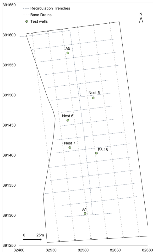
Figure 1. Cell 3 of de Kragge II landfill showing base drains, leachate recirculation system and location of test piezometers.
