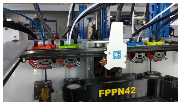
Figure 5.3 E3D tool changer prototype
