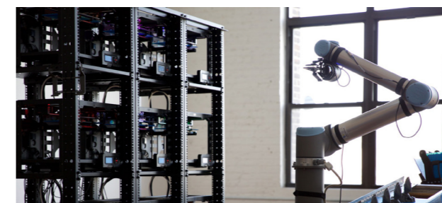
Figure 5.1 Mini factory using 3D printers and a robot arm
