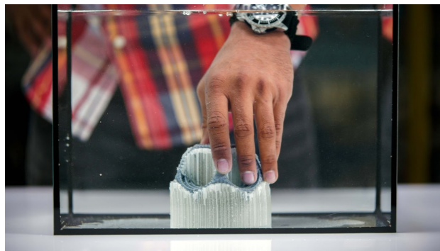
Figure 3.11 Disolvable support material
