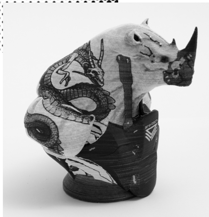
Figure 6.4 Line-based halftoning in material extrusion 3D printing
