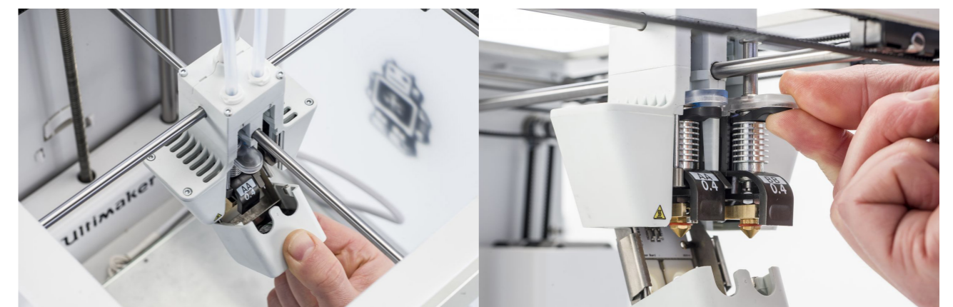
Figure 4.9 Unboxing experience: installing a second print core
