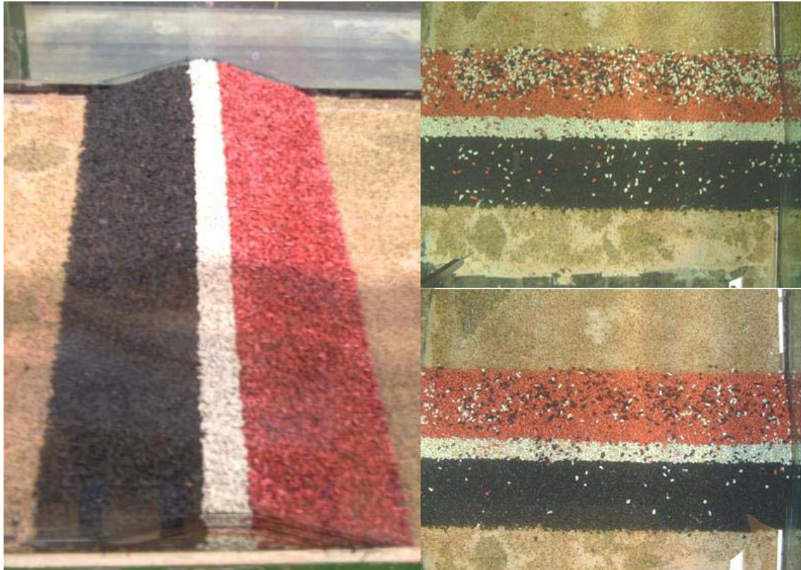
Figure 4-30. A tested structure: on the left the structure before waves. Top right: after 1000 waves. Down right: after 3000 waves
