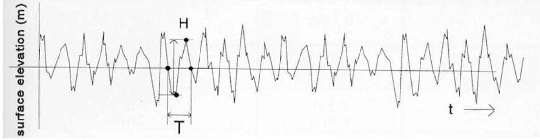
Figure 2-6. A wave signal in time, with registration of zero-down crossings and a defined wave height ( H ) in between
