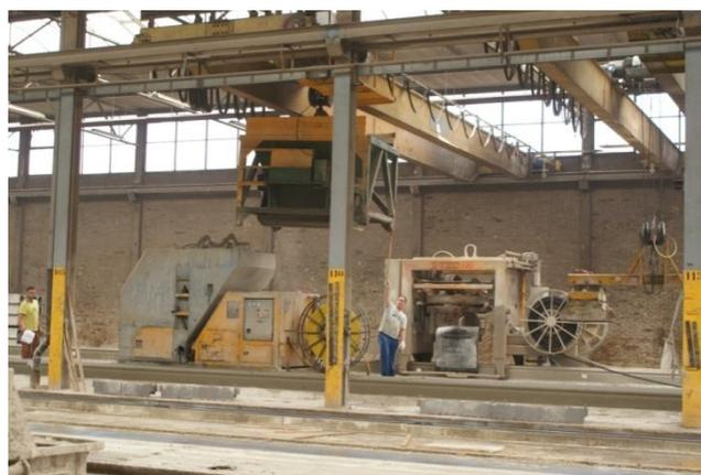
Hollow-core-slabs in production (extrusion)
