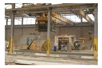
Hollow-core-slabs in production (extrusion)
