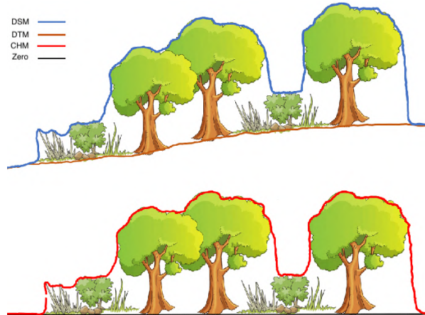
Figure 3.1: Different LiDAR-derived elevation models. The DSM represents the surface elevation, including features such as trees, while the DTM represents the bare ground elevation. The CHM is the resulting height of the vegetation, calculated by subtracting the DTM from the DSM. Source: Jafarbiglu and Pourreza, 2022
