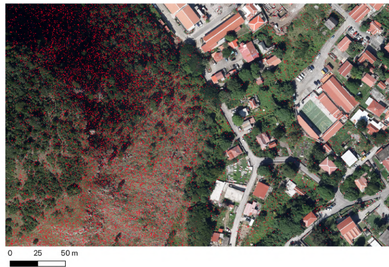
Figure 6.1: A visual overview of pixels for which the lowest elevation of the LiDAR point within that pixel is not classified as ground (indicated in red), zoomed in on an area overlaying the RGB image.
