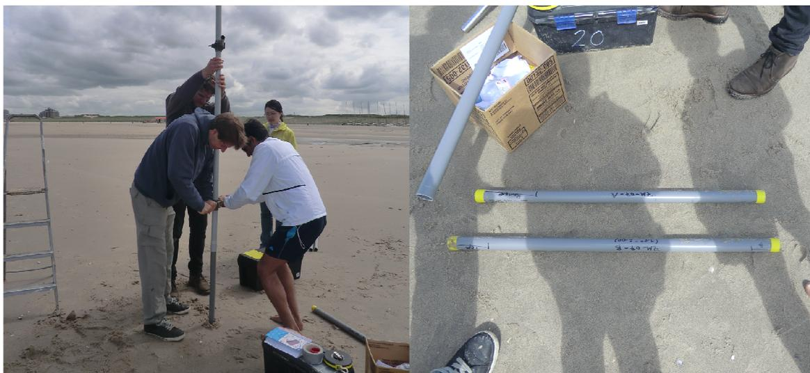
**Figure III-4: Sampling on the Sand Engine using the 'Van der Staay' suction corer. Coring using the corer(left), Samples in light tight containers (PVC-tube)(right).**
