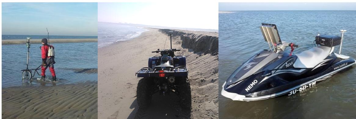
**Figure III-2: Bathymetry measurement equipment (source: Shore Monitoring & Research). Wheelie/Backpack GPS (left), 4wd quad with GPS (middle), Jet ski fitted with GPS and single beam echo sounder (right)**
