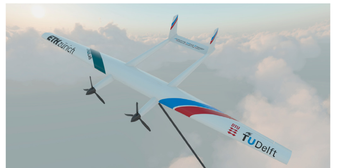
Fig. 7. Rendering of the airborne component of the MegAWES large scale airborne wind energy system.
