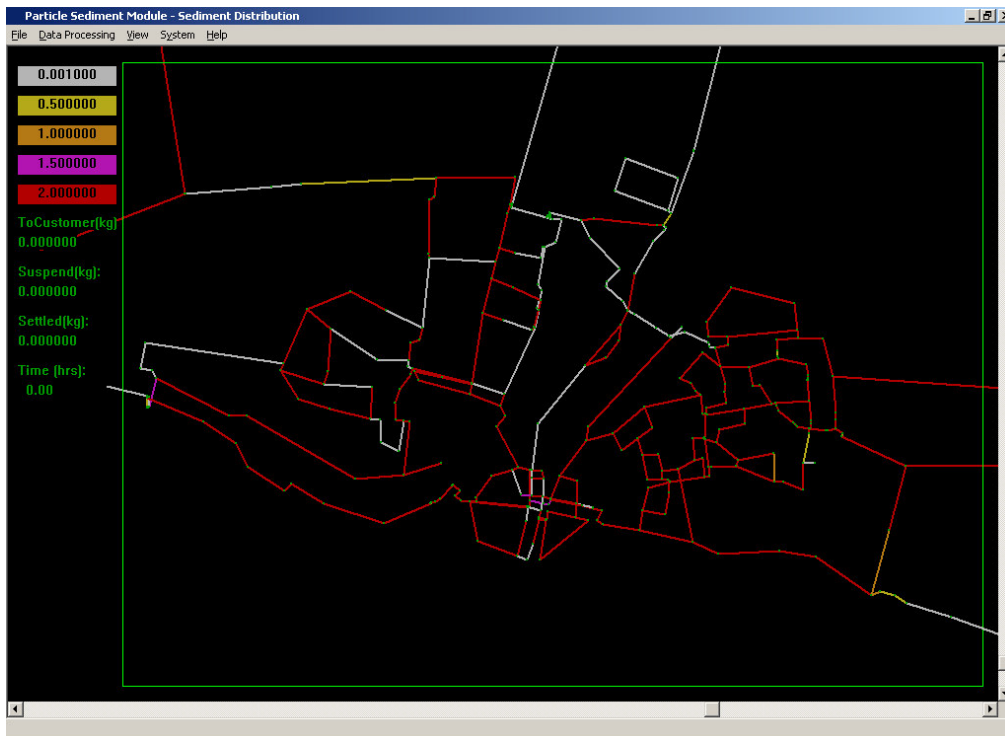
Figure 8-12: Sediment distribution after 1 year, parameters: u_s = 5.5e-6 m/s; u_d = 0.10 m/s; u_{rs} = 0.25 m/s near Gorinchem
