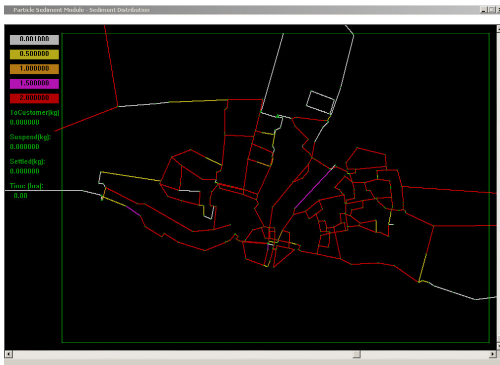
Figure 8-14: Sediment distribution after 1 year, parameters: u_s = 5.5e-6 m/s; u_d = 0.25 m/s; u_{rs} = 0.25 m/s, near Gorinchem
