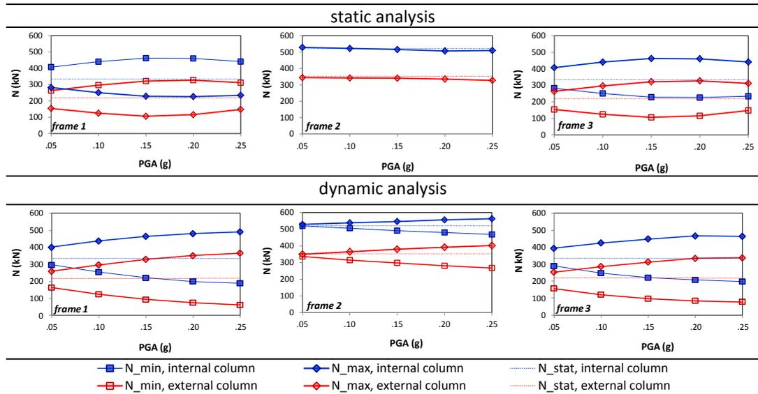
Figure 3. Axial load variation in the columns.
