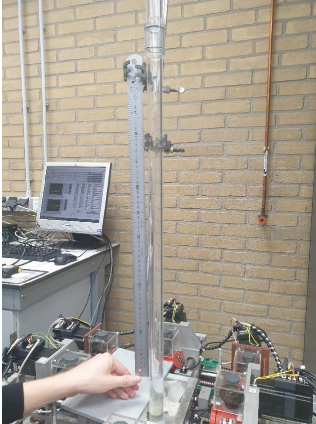
Figure 30: Verification of excess pore pressure measurement using a water column.
