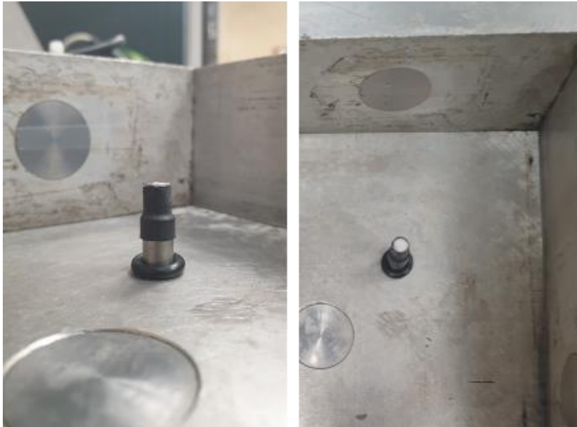
Figure 87: Side view (left) and top view (right) of glass granule placed in biaxial cell.
