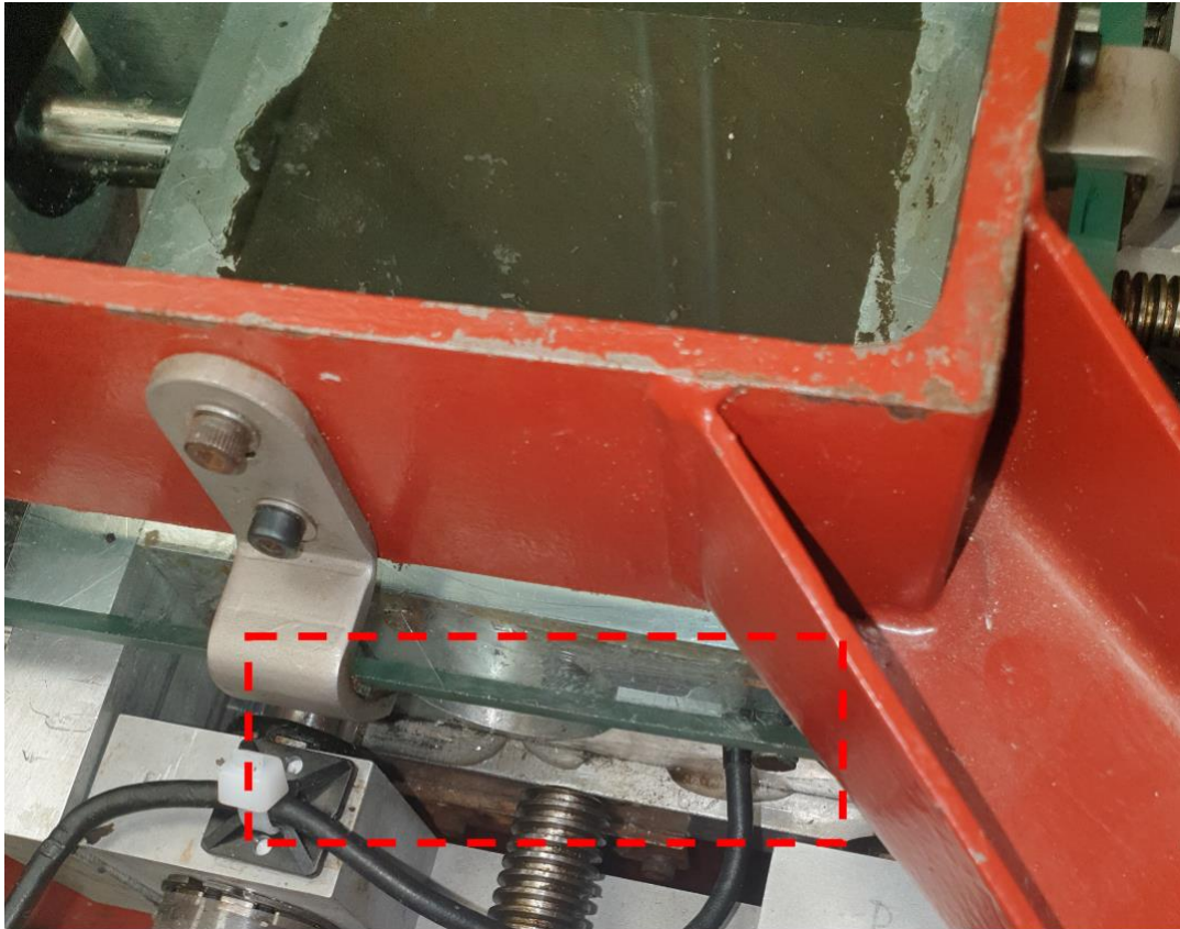
Figure 29: Seepage of water between the bottom plate and vertical plates during biaxial loading.
