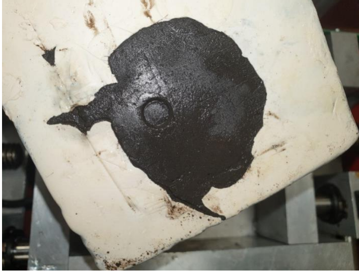
Figure 73: Bottom side of OVP Clay sample covered in latex for T2.
