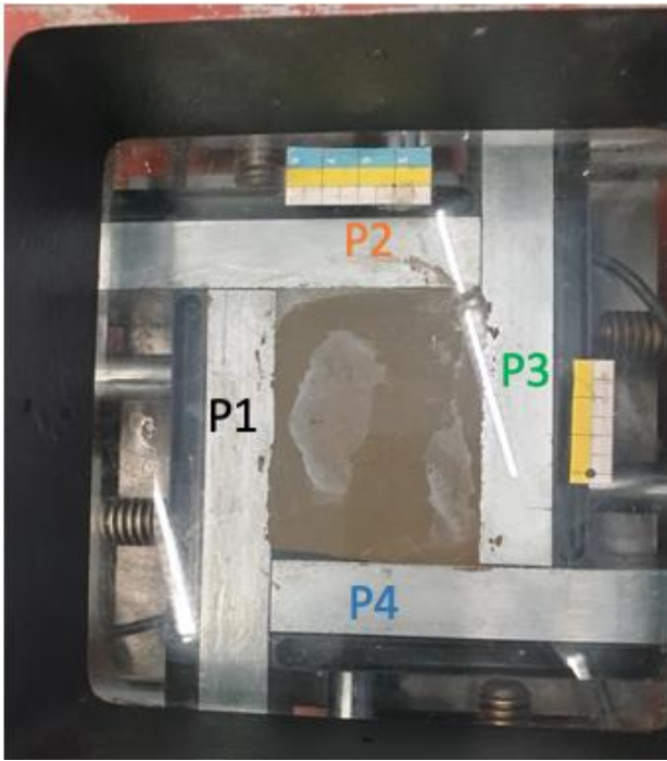
Figure 23: Deformed sample after applying the configuration of Figure 22.
