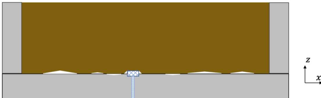
Figure 79: Side view biaxial cell with contact sample and bottom plate discontinued by air voids.
