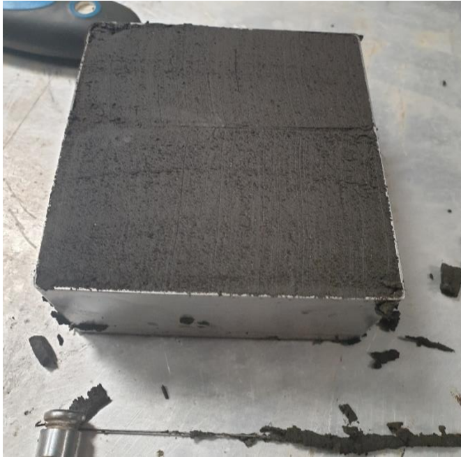
Figure 72: Trimming of OVP clay used for T2.
