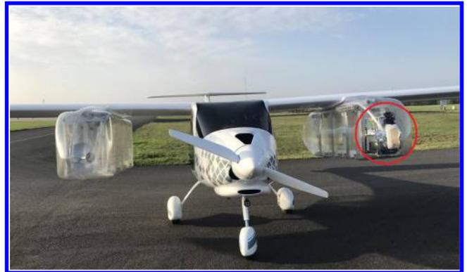
**Fig. 10** The test aircraft, with the radar in the port freight container.
