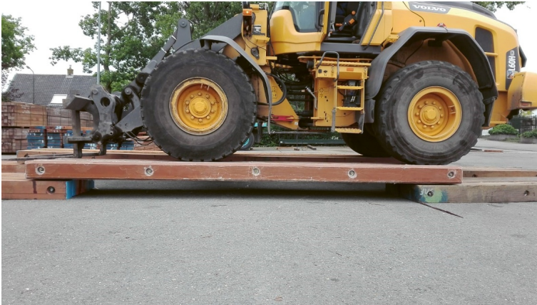
Figure 1.30: Crane mat of EoU composite tested with heavy vehicle (obtained by ten Busschen).
