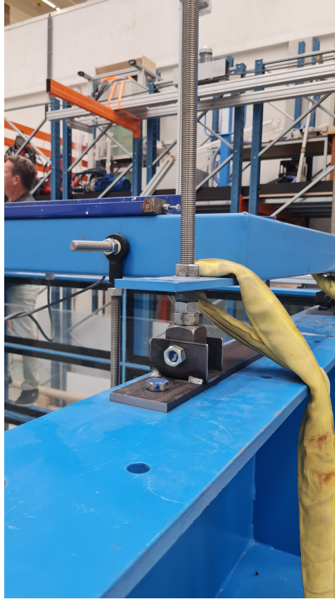
Figure 3.3: Threaded rod, supported by a hinge, to adjust the angle of the rails and table
