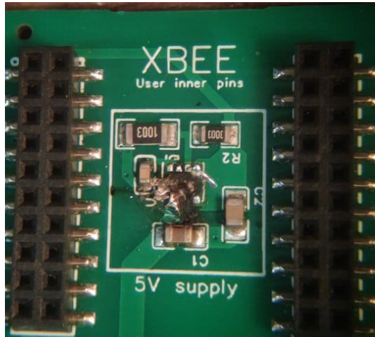
Figure C.2: Photo showing capacitor C1 after plugging the board in.
