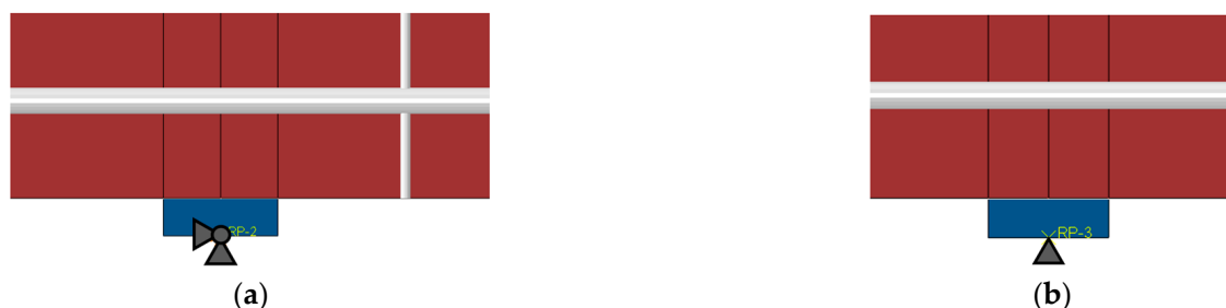
Figure 6. Boundary conditions applied at the supports: (a) left and (b) right of the numerical models.
