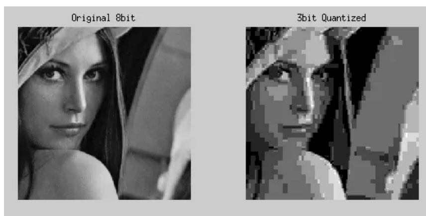
FIGURE 4.1: Example of the effect quantization has on an image (Weksler, 2021).
