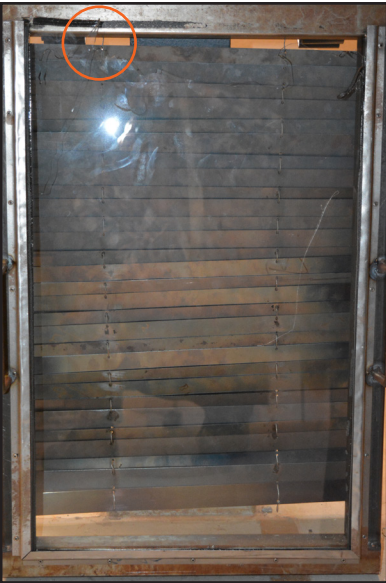
6 mm glass with the closed element at 75 mm distance. Breakage at 89.7 degrees Celsius.
