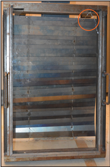
4 mm glass with the closed element at 75 mm distance. Breakage at 70.0 degrees Celsius.
