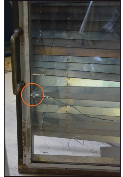
4 mm glass with the open element at 100 mm distance. Breakage at 115.1 degrees Celsius.
