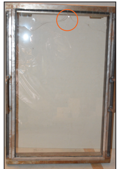
6 mm glass with the closed element at 100 mm distance. Breakage at 36.4 degrees Celsius.
