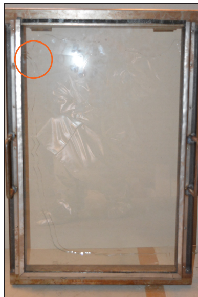
4 mm glass with the closed element at 100 mm distance. Breakage at 55.1 degrees Celsius.
