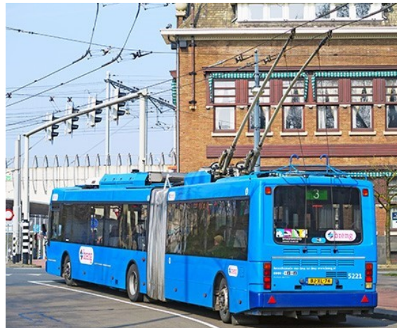
(a) Picture of a trolleybus, powered by overhead wires [5].
