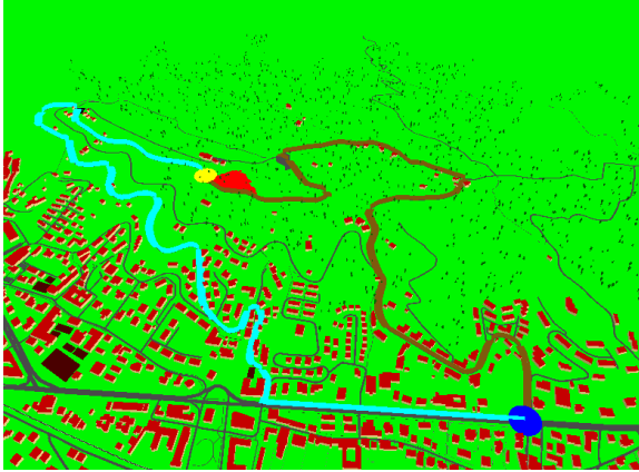
Figure 5: The calculated paths (speed=20 km/h) from the blue point to the yellow point through the environment with one fire-affected area (in red)
