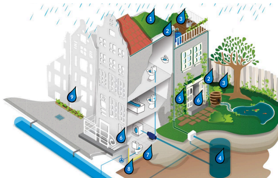
Figure G1: Indication of measures that can be applied around the house. 1: Green roof, 2: Disconnecting Drainpipe, 3: Rain barrel, 4: Rainwater harvesting, 5: Green facade, 6: Elevated doorstep/floor level, 7: water robust cellar, 8: pomp, 9: facade garden. (Amsterdam Rainproof: https://www.rainproof.nl/wat-kan-ik-doen/gebouw )
