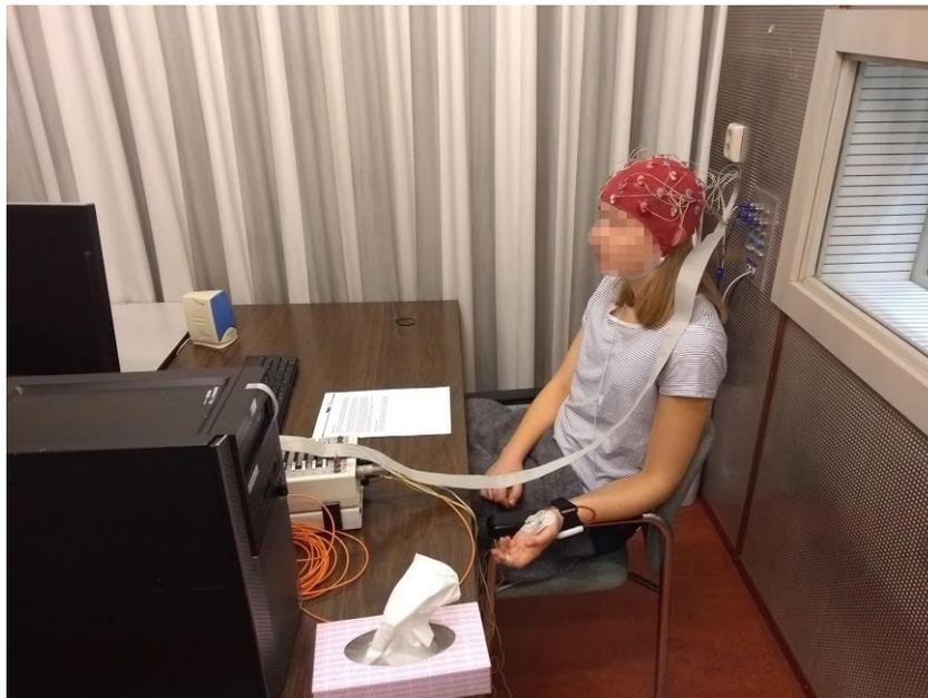
**Figure 2.1** A participant in the experimental setup. EDA sensors were placed on the non-dominant left hand, ECG sensors were placed on the lower left rib and right clavicle and a 32 channel EEG-cap was placed according to the 10-20 system. Audio was played through the white speakers placed in front of the participant.
