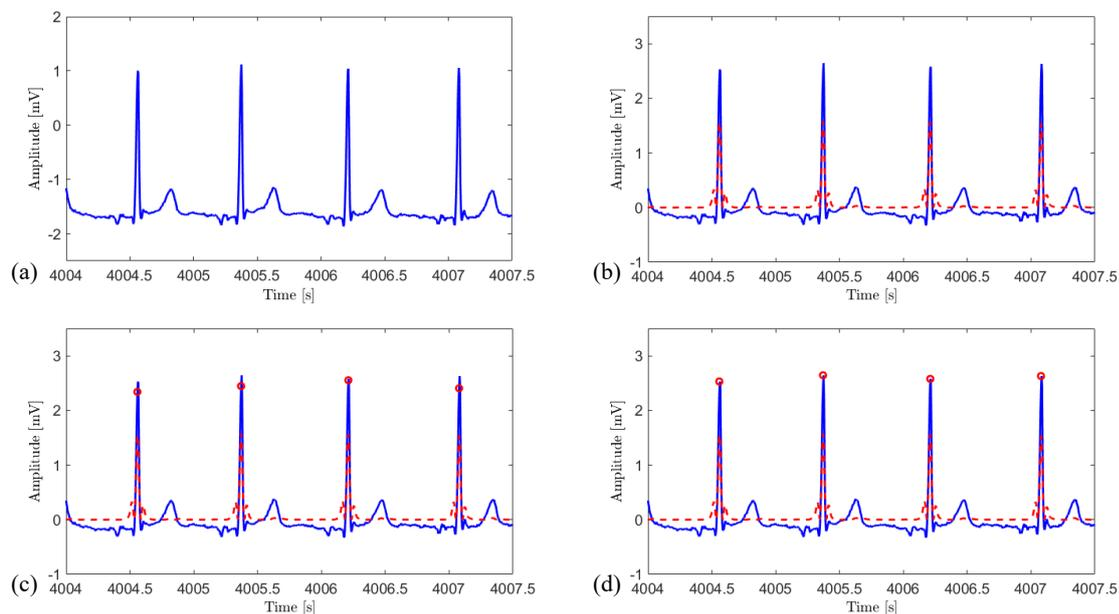
**Figure E.1** Processing steps for ECG peak detection on data from a representative participant. (a) Raw ECG signal. (b) Filtered ECG signal (-) and squared version of the frequency localized reconstructed waveform using wavelet coefficients (-). (c) Uncorrected detection of R peaks (o). (d) Corrected detection of R peaks.
