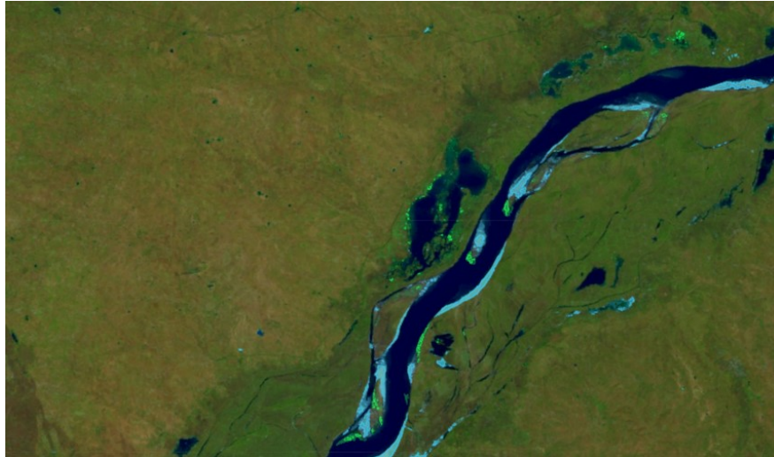
Figure 30 Bank retreat (blue) and accretion (green) in the Ayeyarwady River made visible with the Aquamonitor. The image is the result of a comparison of a reach in the Ayeyarwady River between 2014 and 2016.
