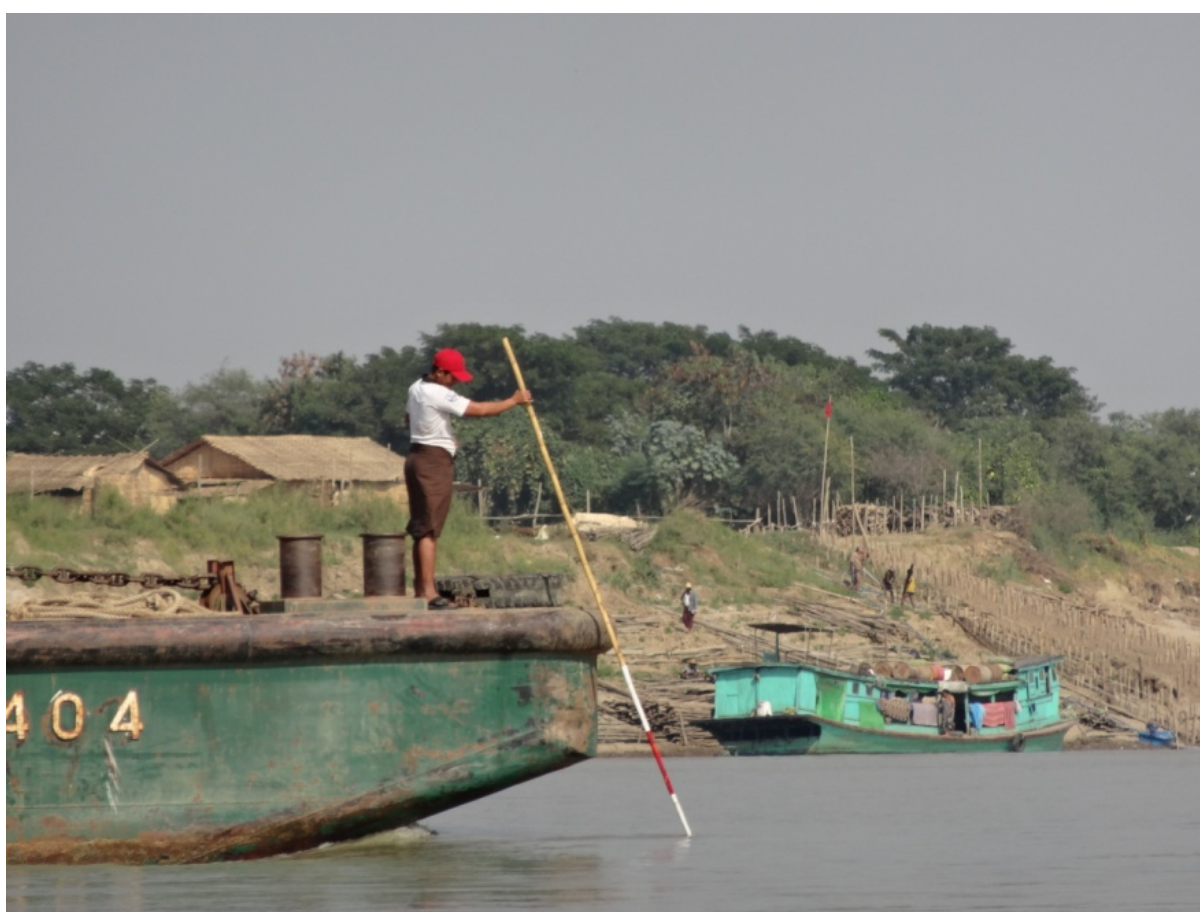
Figure 1 A crew member on a large inland water transport vessel measuring the depth of the Ayeyarwady River with a measuring pole. The ever changing width and depth of the river are a large problem for inland water transport.
