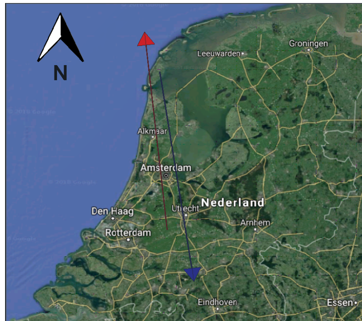
Figure 4.6: Example of satellite ground tracks projected on an aerial photo of Google Maps. In red, the track of the TerraSAR-X satellite is shown in ascending orbit (inclination angle 97.4 degrees). In blue, the track of the Radarsat-2 satellite is shown in descending orbit (inclination angle of 98.6 degrees).
