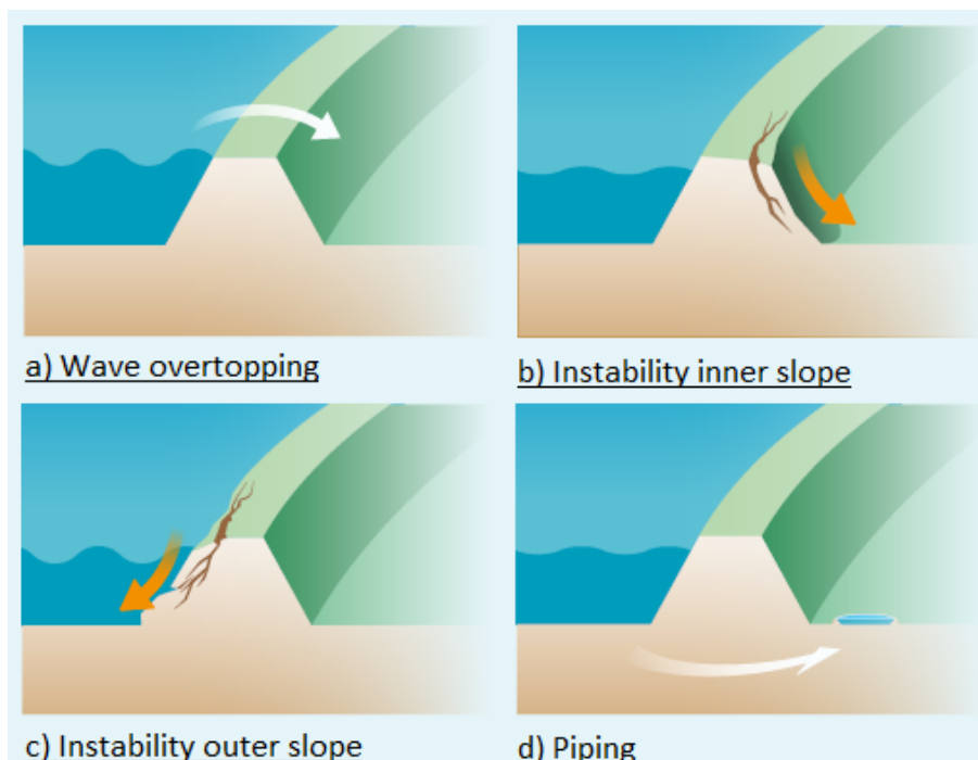
Figure 2.5: The four most common failure mechanisms of dikes in the Netherlands (Vergouwe, 2015) .
