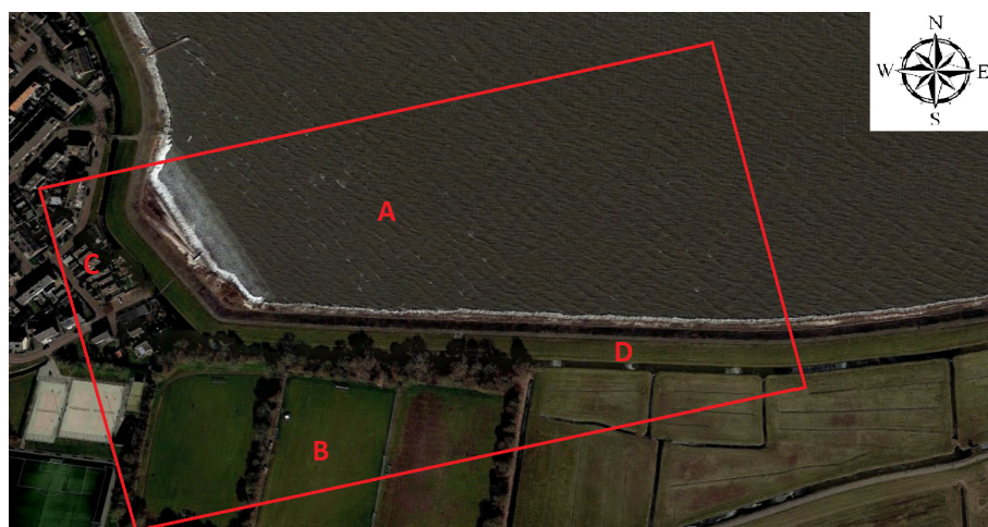
Figure 6.2: Aerial photo of the selected crop (Google Earth). The letters indicate different surface types for which the amount of SHP will be analyzed. A indicates an area on the water surface, B indicates an area on the grassland, C is placed in an urban area and D is placed on the dike itself. The red box approximates the coordinates of the processed cropped radar image.
