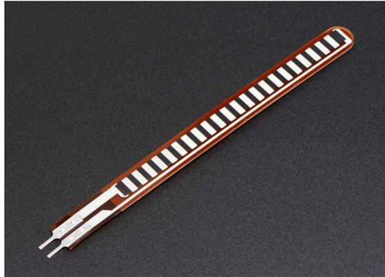
Figure 2.10: Simple resistive strain sensor
