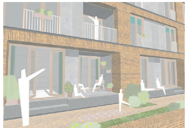
Figure 6: Raised ground floor and extended façade creating a semi-private threshold zone that supports both privacy and informal social interaction (Sumatrahof, Leiden) Source: Platform31 (2021)
