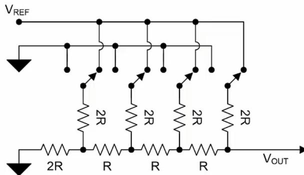
Figure 2: R-2R ladder DAC architecture.
