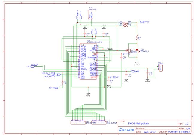
Figure 14: Circuit Schematic (Sheet 4) - DAC 3 in daisy-chain
