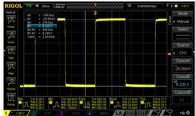
Figure 9: Square-wave output of a single LTC2688 channel (code 2890), expected  $+6.17$  V, measured at  $+6.22$  V with frequency of 992 Hz.
