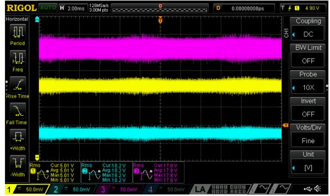
Figure 4: Oscilloscope traces of +17.8 and -18.2 analog rails (pink/blue) and 5.01 V logic rail (yellow).
