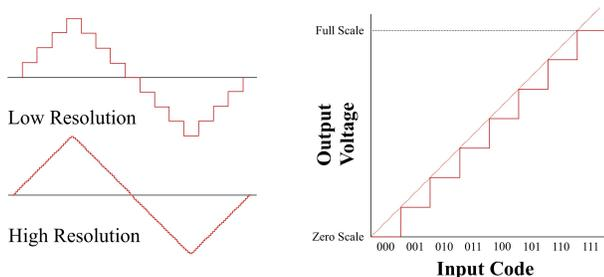
Figure 1: Effect of DAC resolution on output waveform and voltage levels.
