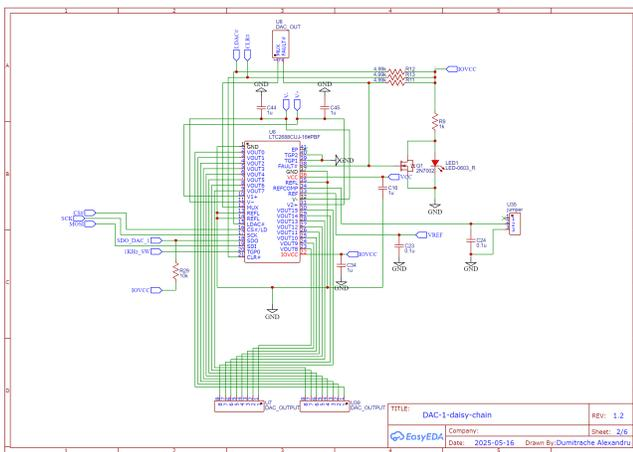
Figure 12: Circuit Schematic (Sheet 2) - DAC 1 in daisy-chain
