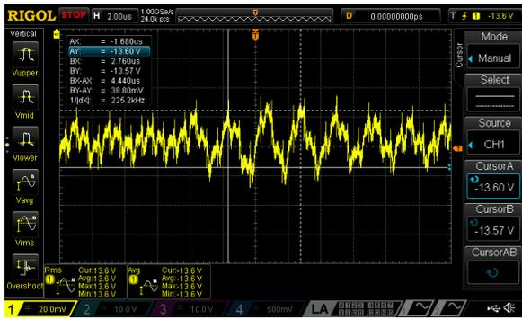
Figure 6: Static output with code 200: expected  $-13.54$  V, measured  $-13.58$  V.
