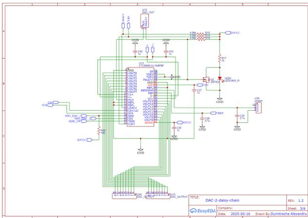
Figure 13: Circuit Schematic (Sheet 3) - DAC 2 in daisy-chain
