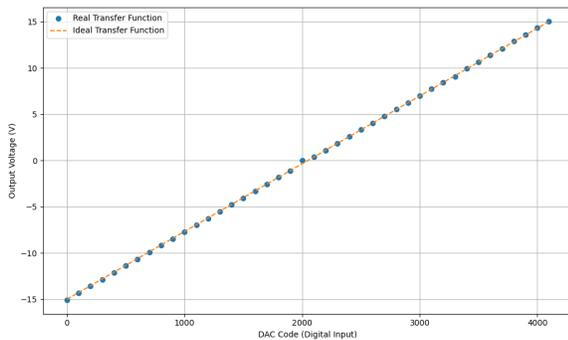
Figure 7: Sampled transfer function (blue) vs. ideal response (orange) for codes 0–4095.
