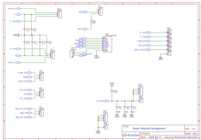
Figure 16: Circuit Schematic (Sheet 6) - Power external management
