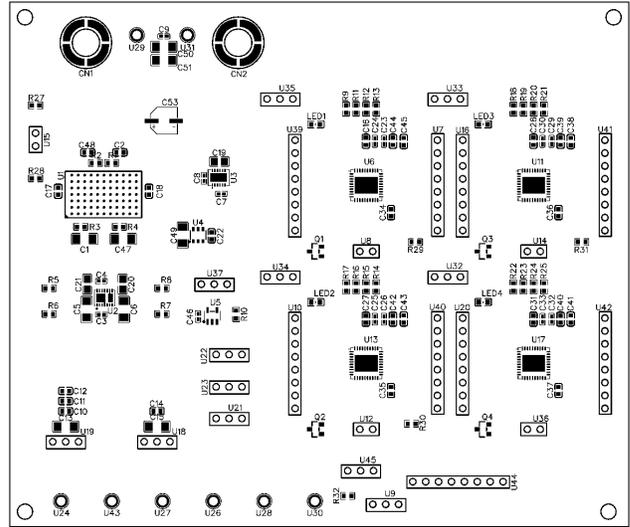
Figure 18: PCB footprint layout indicating the designated placement positions for components such as connectors, integrated circuits, resistors, capacitors, LEDs, and transistors on the board. Each component is labeled with its reference designator to guide accurate assembly.
