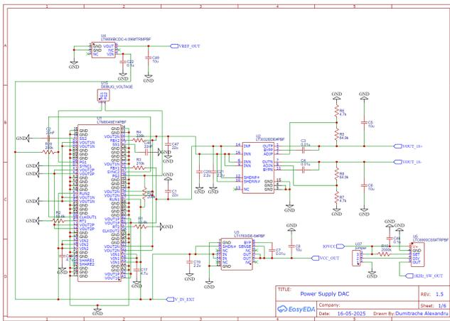
Figure 11: Circuit Schematic (Sheet 1) - Power supply
