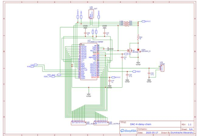
Figure 15: Circuit Schematic (Sheet 5) - DAC 4 in daisy-chain
