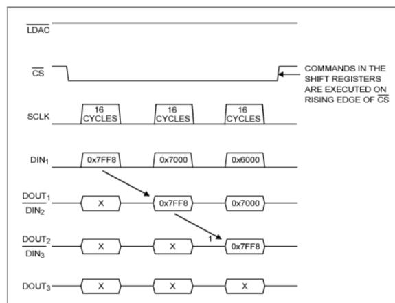
Figure 3: SPI daisy-chain timing for three 16-bit DAC instructions.
