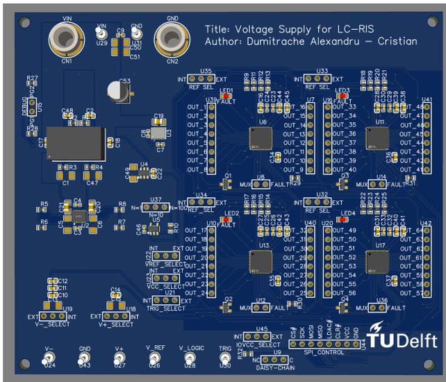
Figure 17: Render of the PCB design of the LTC2688 daisy-chain based system
