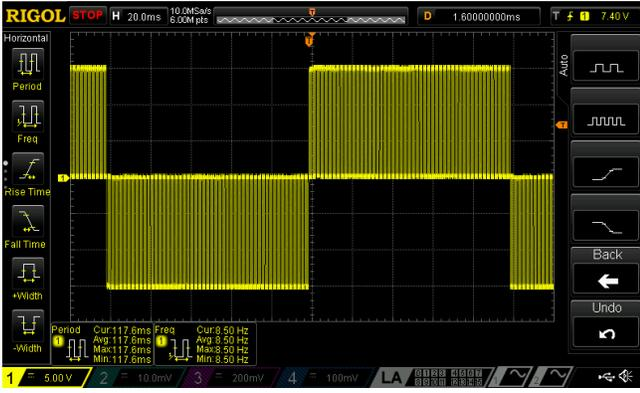
Figure 10: Square-wave output of a single LTC2688 channel, toggling between codes 0 and 4095 every 117.6 ms.
