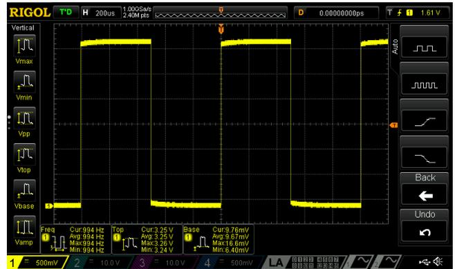
Figure 5: LTC6900 oscillator output (994 Hz).
