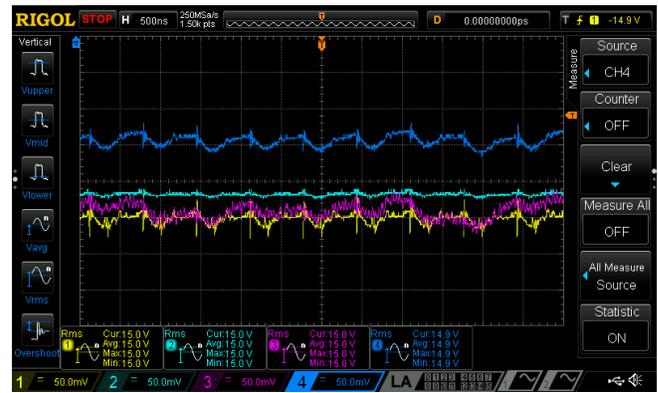
Figure 8: Measured outputs for four LTC2688 devices in a daisy-chain, each set to code 0 (nominal  $-15$  V):  $-15.05$  V (yellow),  $-15.04$  V (pink),  $-15.02$  V (aqua),  $-14.95$  V (blue).
