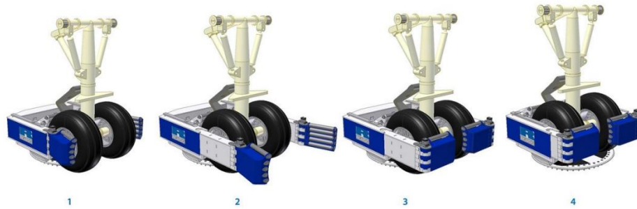
Figure 3.2: Visualization of the working principle of coupling an aircraft nose landing gear to a TaxiBot. Taken from [50].
