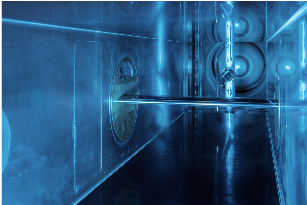
Figure 2.3: Test section of the Cryogenic Ludwig Tube Göttingen 4 . View in flow direction with an unswept wing installed between the vertical walls. In the background, the wake rake and the control valve are visible.
