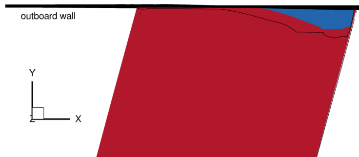
Figure 4.7: Friction coefficient on the wing's suction side at the outboard wall for simulations with two angles of attack. The colormap shows the friction coefficient for \alpha = 0^\circ , where red indicates regions with positive friction coefficient, and blue indicates regions with zero or negative friction coefficient. The black line indicates the line of zero friction coefficient for \alpha = 2^\circ . The simulations are performed for \Lambda = 15^\circ, c = 150 \text{ mm}, Ma = 0.65 , and Re = 7 \times 10^6 .
