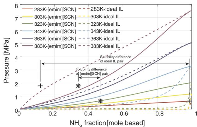
**Fig. 10.** Comparison of the P-T-x behavior between the optimized NH<sub>3</sub>/IL pair and the real pair (NH<sub>3</sub>/[emim][SCN]).
