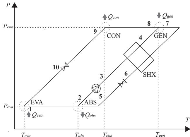
Fig. 2. The single-effect AHP cycle on a  $\ln P - (-1/T)$  diagram.
