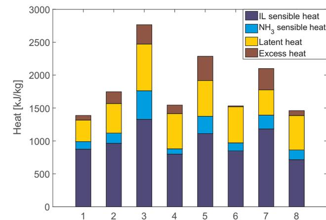
**Fig. 6.** Contributions to the GEN heat  $Q_{gen}$  by the 4 terms of Eq. (16). The 4 terms are latent heat, absorption heat and sensible heats of both components. 1–8 denotes NH<sub>3</sub> based working fluids with [mmim][DMP], [emim][BF<sub>4</sub>], [omim][BF<sub>4</sub>], [bmim][BF<sub>4</sub>], [bmim][PF<sub>6</sub>], [emim][Tf<sub>2</sub>N], [emim][EtSO<sub>4</sub>] and [emim][SCN].
