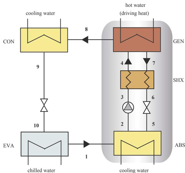
Fig. 1. Schematic diagram of a single-effect AHP system using IL based working pair.
