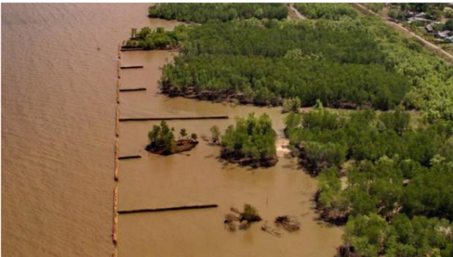
Fig. Wave dampening effect of bamboo T-fences, Ca Mau Province, Viet Nam Photo: R. Sorgenfrei 2016
