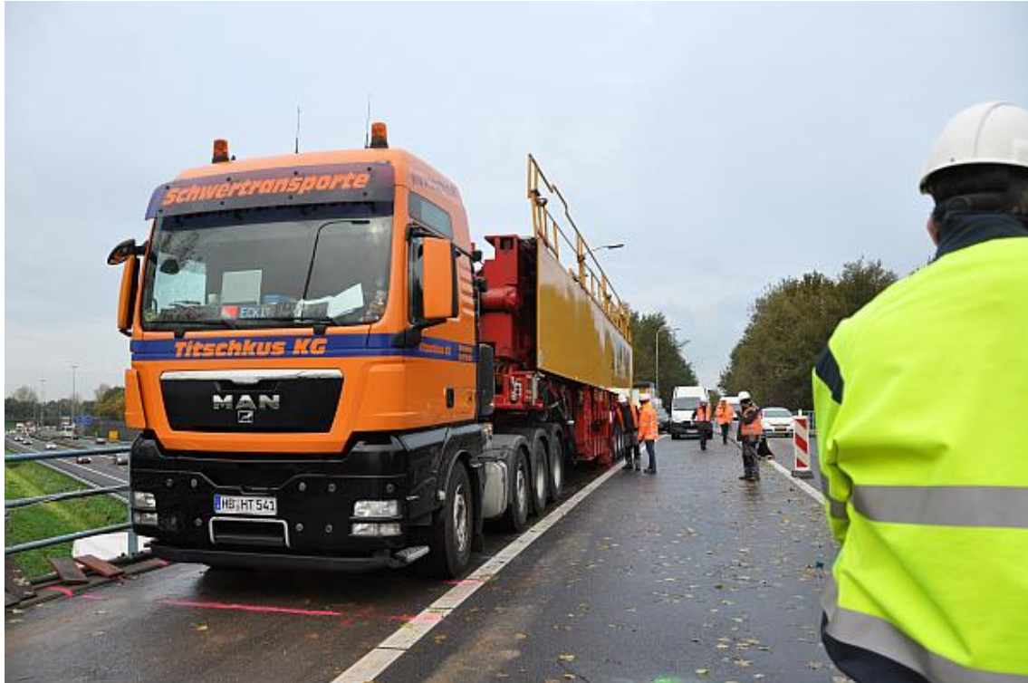
Figure 1. Example of special loading vehicle. Photograph by D.A. Hordijk, used with permission.
