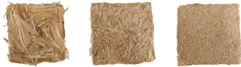
Starch binder 8 g starch - 80 ml Water 50 mm fibers 15 g Starch binder 8 g starch - 80 ml Water 15 mm fibers 15 g Starch binder 8 g starch - 80 ml Water 5 mm fibers 15 g
