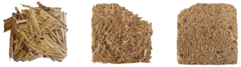
Tannin binder 8 g starch - 16 ml Water - 0.7 g lime 50 mm fibers 15 g Tannin binder 8 g starch - 16 ml Water - 0.7 g lime 15 mm fibers 15 g Tannin binder 8 g starch - 16 ml Water - 0.7 g lime 5 mm fibers 15 g
