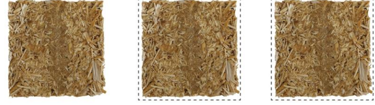
(Bio) Epoxy binder 3 g epoxy resin - 1 g hardener 50 mm fibers 15 g (Bio) Epoxy binder 3 g epoxy resin - 1 g hardener 15 mm fibers 15 g (Bio) Epoxy binder 3 g epoxy resin - 1 g hardener 5 mm fibers 15 g
