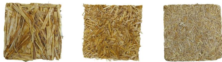
Casein binder 8 g casein - 18 ml water - 0.8 g lime 50 mm fibers 15 g Casein binder 8 g casein - 18 ml water - 0.8 g lime 15 mm fibers 15 g Casein binder 8 g casein - 18 ml water - 0.8 g lime 5 mm fibers 15 g
