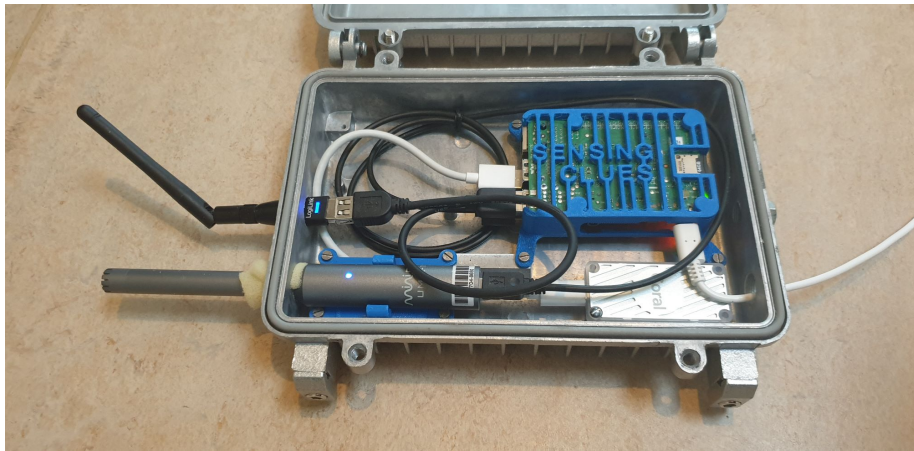
Figure 6.1: An opened OpenEars device with the Coral TPU added
