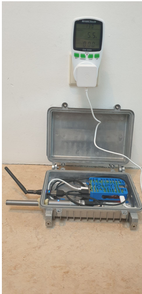
Figure 6.3: The setup for measuring power consumption. A Basetech EM-3000 is placed between the power outlet and the Raspberry PI power adapter, measuring power usage of the device.
