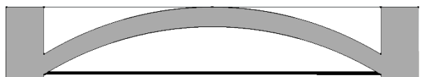
Figure 5.32: The arch beam, first considering compression forces and then adding tensile element
