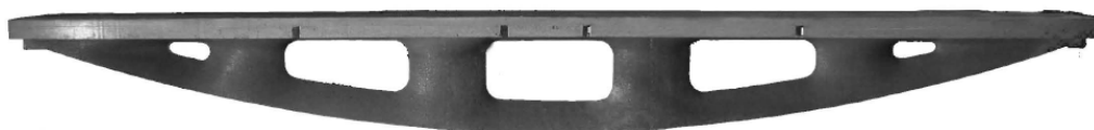
Figure 5.45: Concrete beam casted into textile formwork designed with topological optimization in ANSYS [C.A.S.T. Manitoba University ,Canada]
