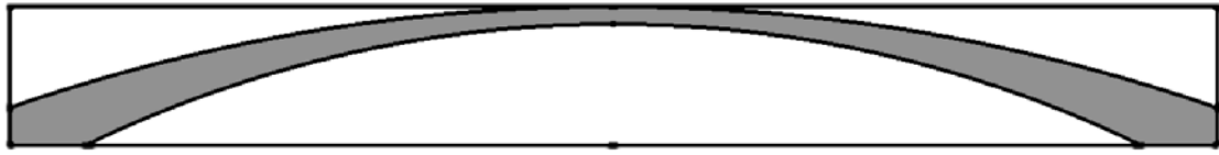
Figure 5.81: Side-view arch beam
