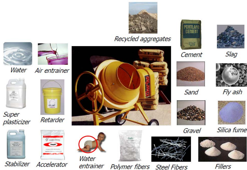
Figure 2.1: Current practice of mixing concrete [Erix Schlangen, 2012]
