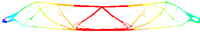
Figure 5.91: Topological optimizations, the colours are indication of the stress levels in each element.
