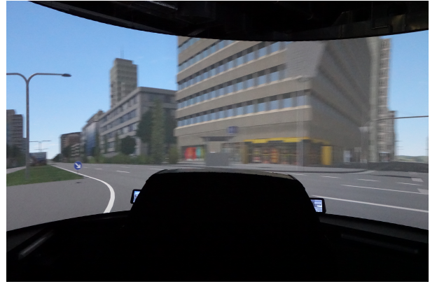
Fig. 16. Visible field of view of a corner seen from behind the simulator motion cabin.
