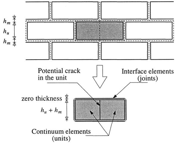
Fig. 3. Suggested modeling strategy. Units ( $u$ ), which are expanded in both directions by the mortar thickness, are modeled with continuum elements. Mortar joints ( $m$ ) and potential cracks in the units are modeled with zero-thickness interface elements.
