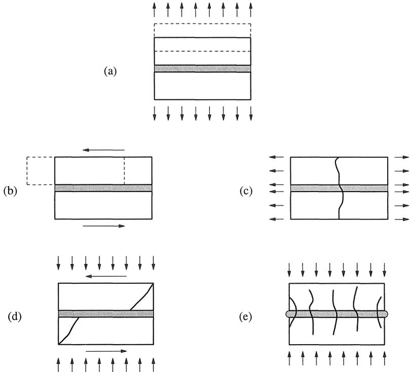
Fig. 2. Masonry failure mechanisms:
