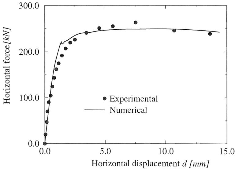
Fig. 16. Wall W. Load - displacement diagrams.
