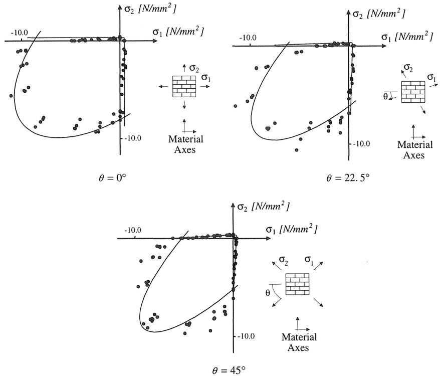
Fig. 13. Comparison between the plasticity model and experimental results from Page (1981,1983).
