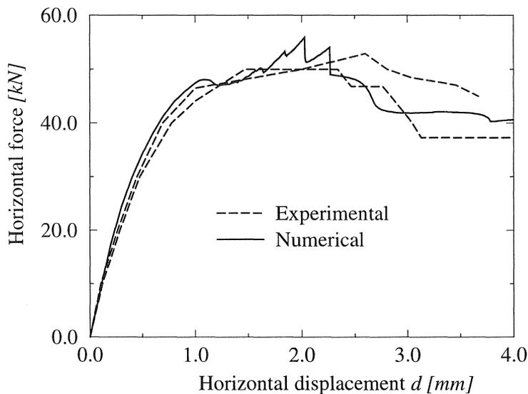
Fig. 8. Wall JD. Load – displacement diagrams.
