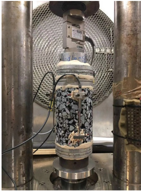
Fig. 9. Uniaxial cyclic compressive tests for PA mixes.
