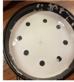
b. Mould for making mortar specimens
