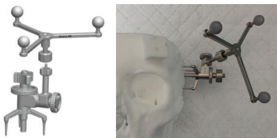
Figure 3.8.: Brainlab's reference star to track the patient.
