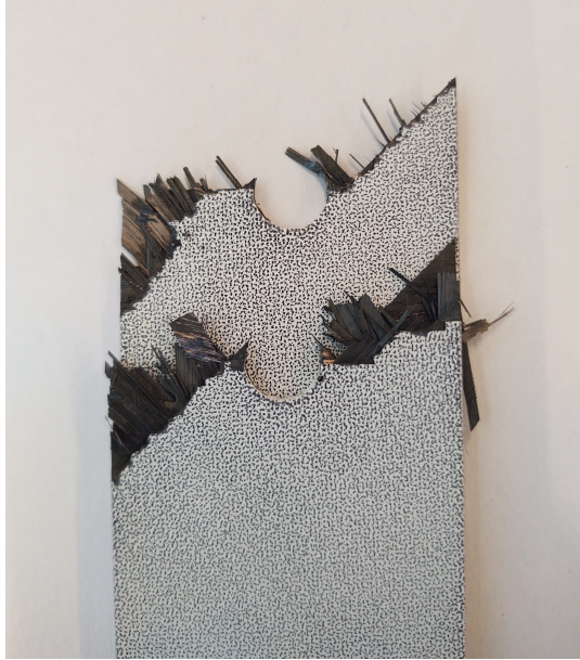
Figure 5.1: Typical static failure (sample 16)
