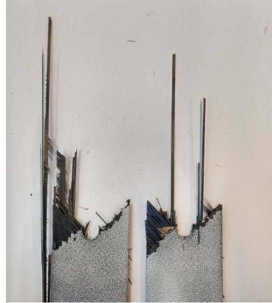
Figure 5.2: Typical fatigue failure (sample 14)
