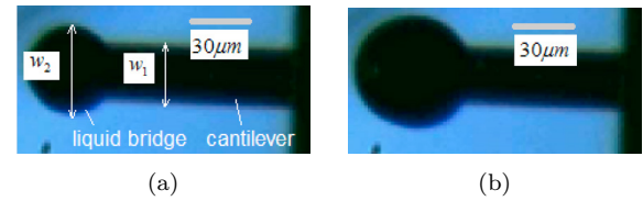
Fig. 10. The dispensing process for small tip-substrate distance. a) Initial image when dispensing started ( t=0 ) b) Final image when dispensing saturated ( t=13 s).
