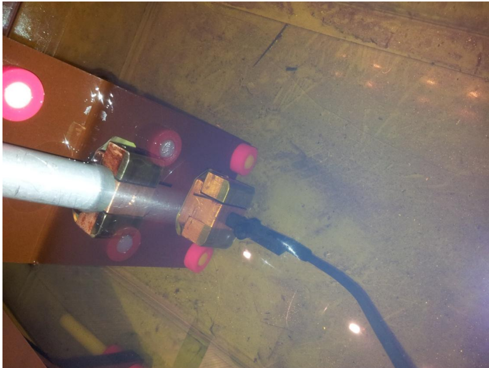
Figure 4.8. The small scale set up put inside transformer oil.
