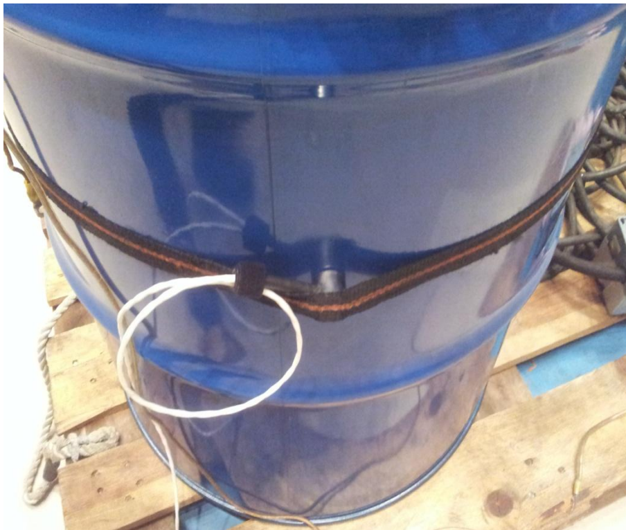
Figure 5.16. Acoustic sensor attached to the metallic enclosure.
