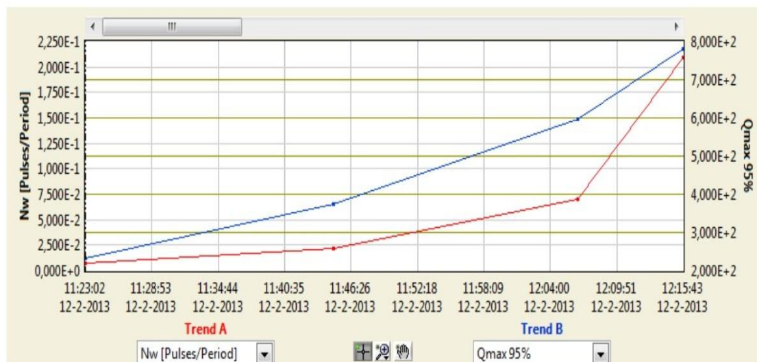
Figure 4.27. The trending of the PD pulses over time and applied voltage.
