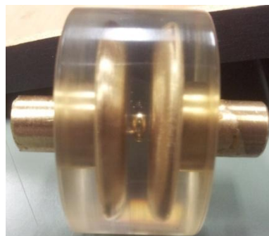
Figure 4.40. Gas bubble in epoxy resin.
