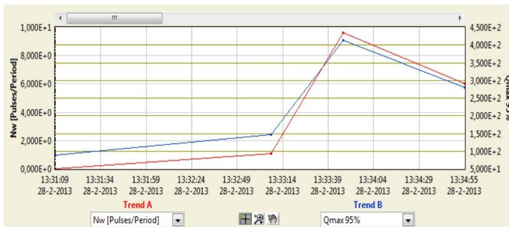
Figure 4.39. Trending of the PD pulses.
