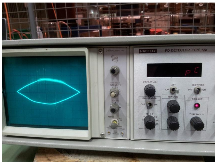
Figure 4.1. Haefely 561 PD detector.
